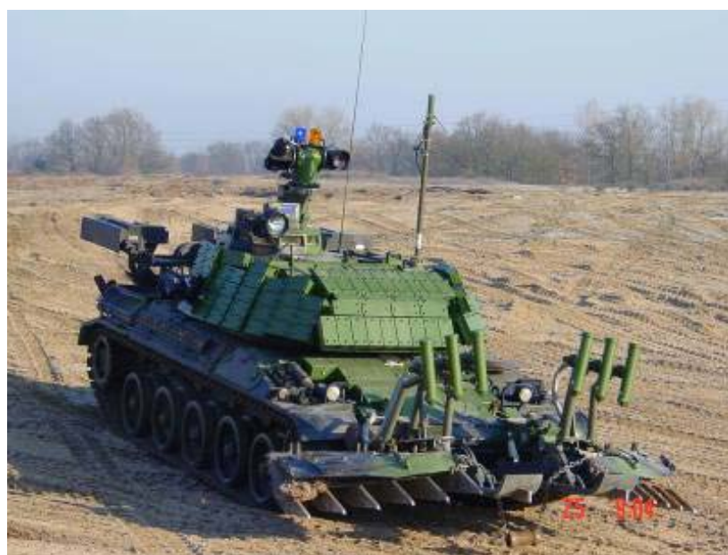
Figure 4-9: Cybernetix “AMX30B2” De-Mining Tank, Tele-Operated (French MoD via Giat Contract).
