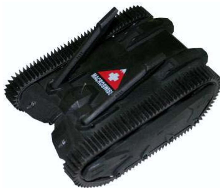
Figure 4-3: Macroswiss “Crawler” Featherweight All Terrain UGV (under 20 cm length and 400 gr weight).
