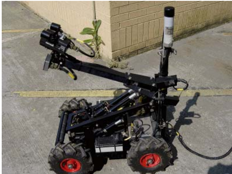
Figure 4-4: “Groundhog” Lightweight Inspection UGV Currently in Service with UK Forces.
