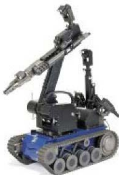
Figure 4-8: Telerob “Teodor” Medium Weight UGV for Interventions in Hostile Environments.
